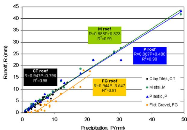
**Fig. 2 – Regression model for roof runoff and rainfall height. Regression equations and corrected  $R^2$  are also shown. Each point represents a rain event.**
