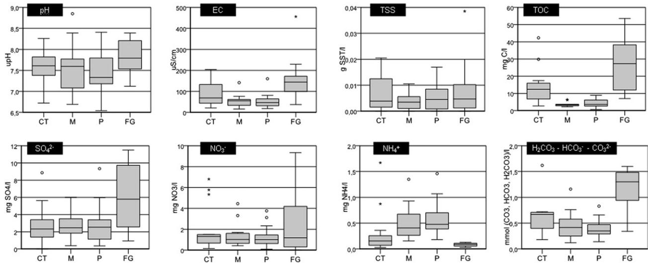
**Fig. 3** – Box plot diagram of rooftop runoff water quality for each roof. Abbreviations: CT = clay tiles; M = metal; P = plastic; FG = flat gravel.
