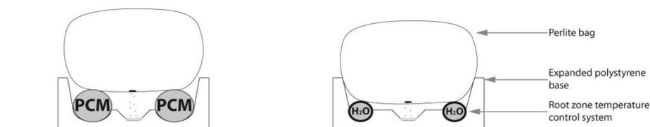
Figure 1. Left: Scenario A PCM application for root zone temperature control. Right: Scenario B oil dependent conventional root zone heating system with hot water scenario.
