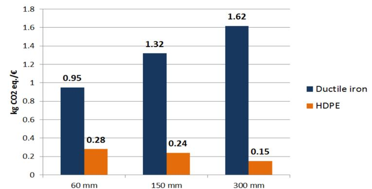
Figure 4. Representation of the indicator kg of CO<sub>2</sub> per € for different pipe sizes.
