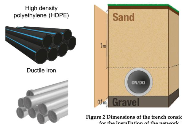
Figure 2 Dimensions of the trench considered for the installation of the network. [5]
