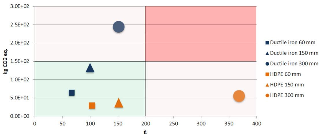
Figure 3. Graphical representation of eco-efficiency results for HDPE and ductile iron pipes constructive solutions of 60, 150 and 300 mm pipe sizes
