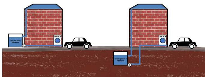
Figure 1. Tank installation diagram. Left: ground level; Right: Underground
